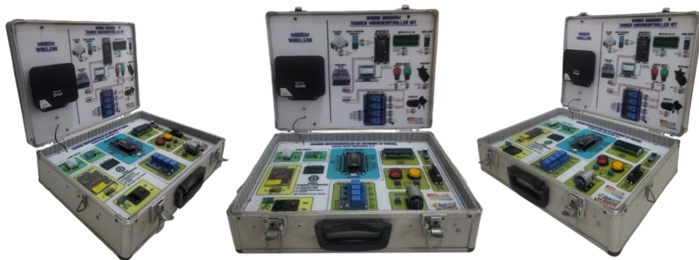
Figure 3. ESP8266-Based IoT training kit design
